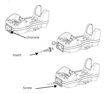
To disconnect the multi-interface cable, open the front door, pull out the cable and screw the front door back.
