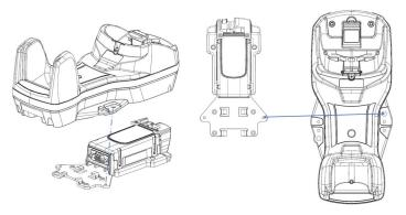
7. Move the base station up until the sphere is aligned with the smaller hole, then lock the lever to secure the connection module.
