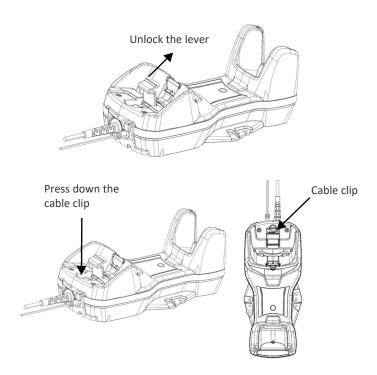
Pull out the multi-interface cable and put the lever back into lock position.
