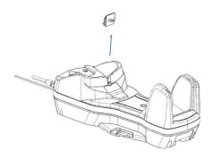
3. Rotate the tab until you will see "WALL" tooth, put the rotated tab into place and secure it with the screw.
