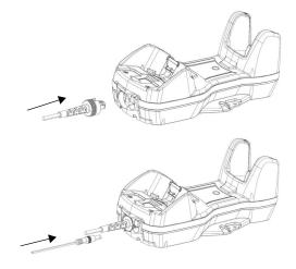
After connecting the power supply cable, secure it on the strain relief as shown in the figure below.
