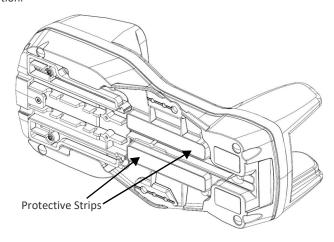
3. Align the base station with the mounting plate until you see the sphere inside the bigger hole on the left.
