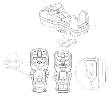
Move the base station down until the sphere is aligned with the smaller hole.
